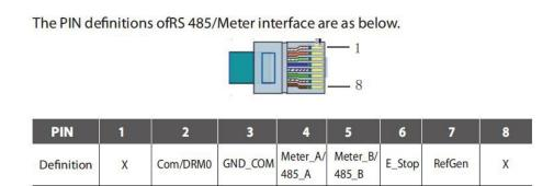
The RS485 data transfer is a differential system with two data lines A and B. (Pin 4 and 5 on the RJ45 plug) They are not grounded to be more resistant to interference. If line A is 5 volts, line B is 0 volts and vice versa. In our system, a MAX 485 module, connected to our Arduino microprocessor, converts the data stream into TTL with 5 volts relative to ground.
