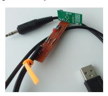
**Transmitter** (left) connected to the 5V and GND of the |Arduino, the angled data header pin is straightened to evade the female header of the Arduino and is lead to digital output 10 at the other side.
