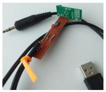
**Transmitter** (left) connected to the 5V and GND of the |Arduino, the angled data header pin is straightened to evade the female header of the Arduino and is lead to digital output 10 at the other side.
