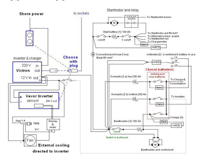
In the morning, before the sun can start charging and after an evening with the use of TV, lights and possibly the heater, the battery voltage is usually at its lowest. Especially after a few days with little sun, the voltage can have dropped quite a bit. If one sails away at such times, it is wise to avoid the use of the bow thrust-er, windlass or other large users, if possible.
