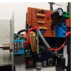
Not pushed in yet to make the pins visible -The two pins to the right are just for mechanical support and are not connected.
