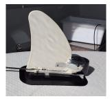
The same transducer mounted together with a plastic fin on a nylon block which slides in the rails at the bottom of a SUP board. Approx 5 cm has to be added to get SDDBS
