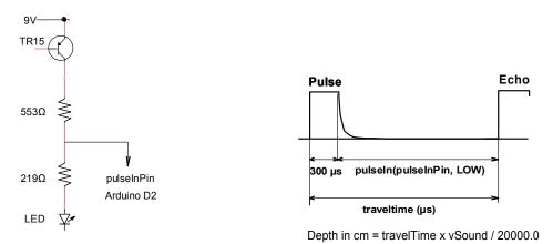
For a vSound in m/s and travelTime in  $\mu$ s, the Depth in cm is: travelTime x vSound / 20000.0 The speed of sound in water, vSound = 1480 m/s
