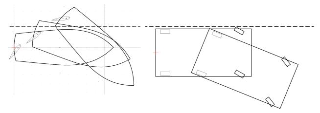
Please note that there must be **enough room at the stern** to turn a ship. This is clearly different from a car, where a steering action moves the **front** sideways
