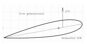
In the case of large shipbuilding, larger than 20% balance percentages are used, but larger forces play a role that one wants to avoid and heavy hydraulic steering machines are used to control a rudder. Also specific tank test and/or computer simulations are carried out beforehand.
