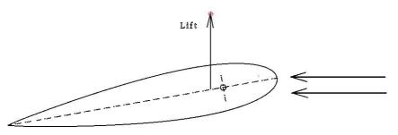
When steering, the rudder blade is put at a certain angle with the passing water. The moving water will cause a lateral force. Similar as with airplane wings, one speaks of lift. The force will depend on the **angle** of the rudder and the **speed** of the passing water. This lateral force pushes **the stern** sideways. This changes the direction (the course) of the vessel.
