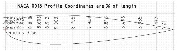
See also: "2023 01 27 Symmetric NACA 0018 Dimensions.pdf" (2 pages) at the downloads page for a calculation example and a blank profile shape to put your own dimensions on.
