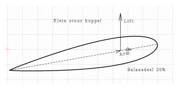
Without specific computer simulations or tests, I would not choose a larger balance part than 20% for small vessels. The mentioned (lift) distance of (0.25 x length), is after all a measured value and concerns a test set-up with an even flow. This is not necessarily equivalent to the actual situation. The propeller for example, rotates at a short distance in front of the rudder.
