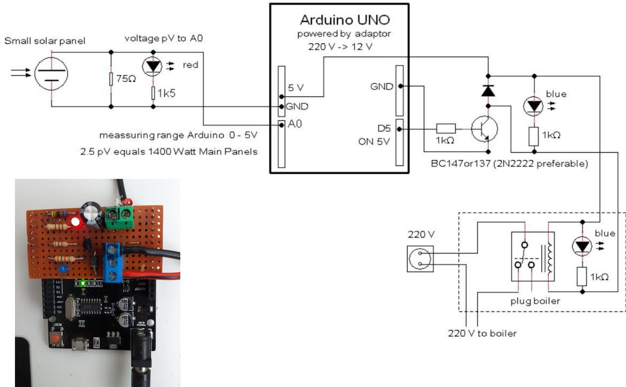
The analogue input of the Arduino microcontroller can handle 0 - 5 V. Therefore the maximum pV is adjusted in order not to exceed 5V. A red LED light will show when the pV reaches 1.8 Volt. In this situation, the main panels deliver 1000 Watt. When digital output D5 triggers the relay of the boiler's socket, the blue LEDs on the print and in the sockethousing light up.
