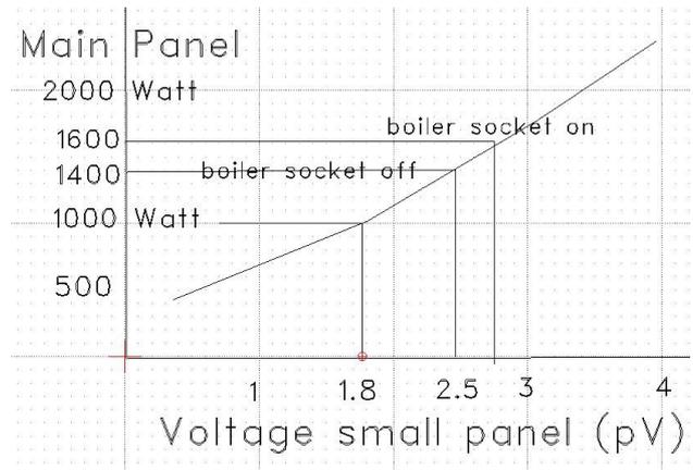
This method needs some re-adjusting during the different seasons. Using the data of the inverter is the most accurate source of course.
