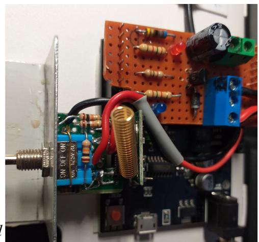
The 10 k pull-down resistors from D10 and 11 to GND are visible on the setup to the right.
